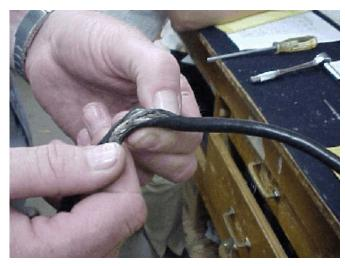
Pictured is a power cord for a shop appliance. The cord has been sliced open, exposing the energized wires. The appliance was still plugged in and still in use.
