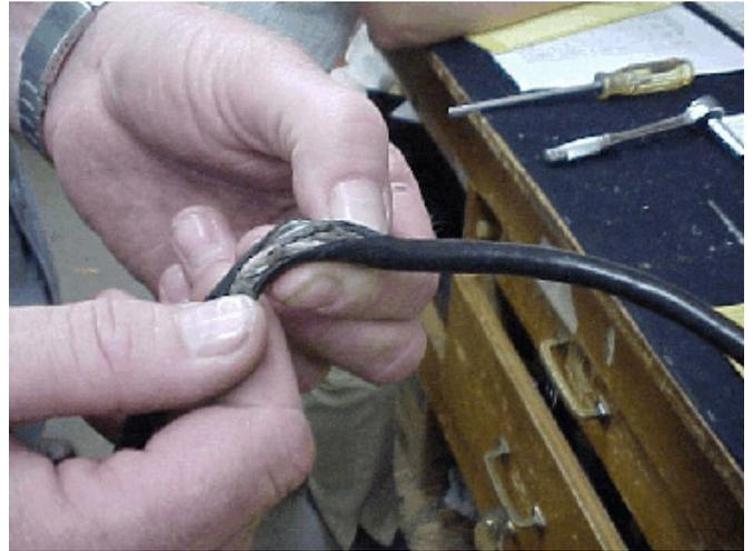
*Pictured is a power cord for a shop appliance. The cord has been sliced open, exposing the energized wires. The appliance was still plugged in and still in use.*
